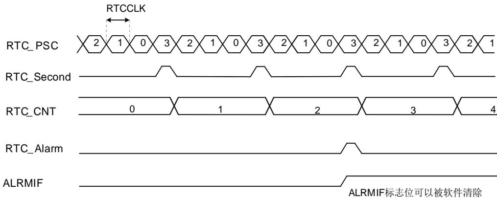
图 14-3. RTC 秒信号及溢出信号的波形(RTC\_PSC = 3)
